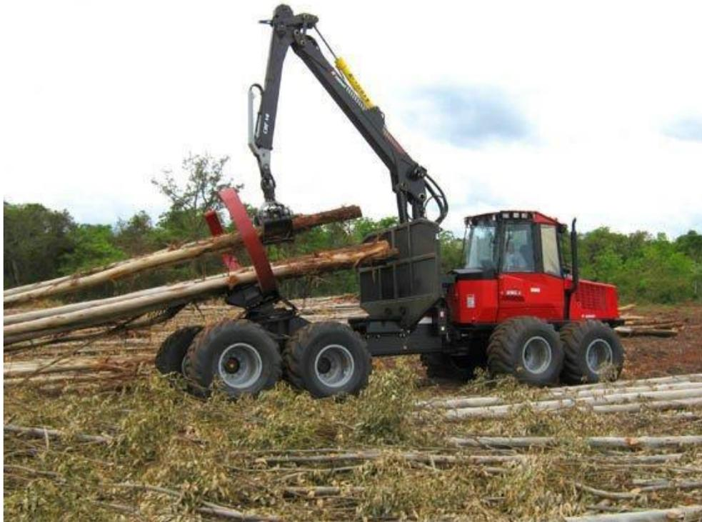
Figura 20: *Clambunskidder* Komatsu 890.3.
