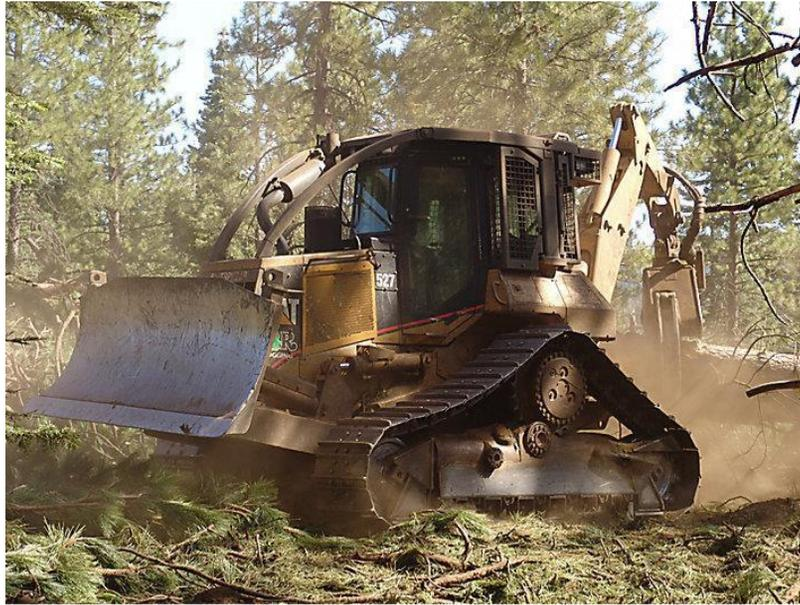
Figura22: *Trackskidder* caterpillar 527.
