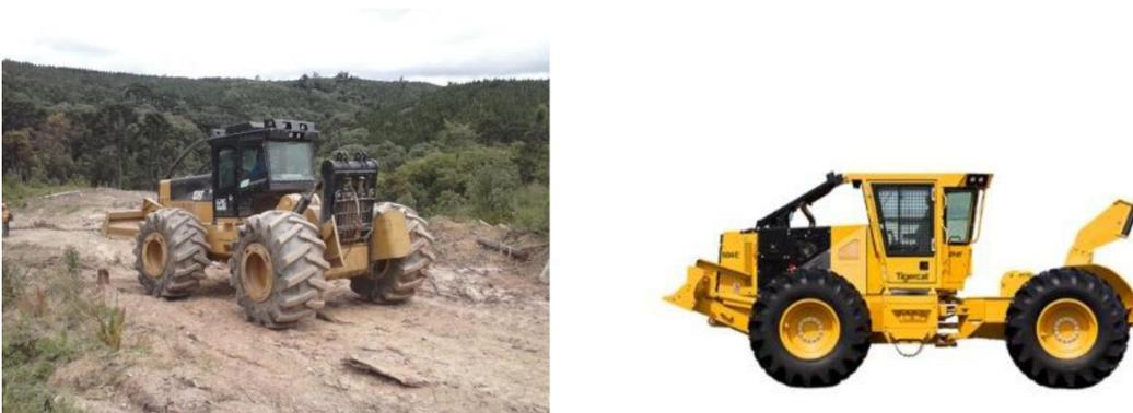
Figura19: Chockerskidder Caterpillar545C e Tigercat 604E.
